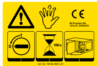
Typical CE label for air handling units
