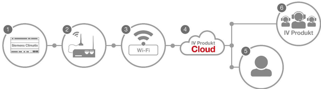
The 4G router (2) is connected to Climatix (1) inside the unit and to the existing network (3). Users (5) or IV Produkt support (6) can then access the unit through IV Produkt Cloud (4).
