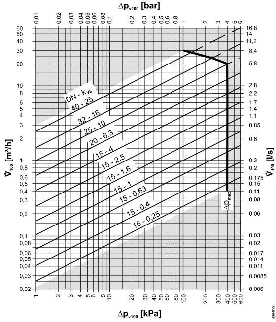
$\begin{array}{lll} \Delta p_{\text{max}} & = & \text{Maximum permissible differential pressure across the valve} \\ & & (\text{VXG44...: mixing port: Ports A-AB, B-AB, diverting: Ports AB-A, AB-B),} \\ & & \text{valid for the entire actuating range valve-actuator unit} \end{array}$
