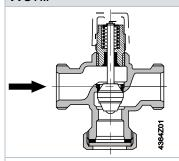
Guided parabolic plug, integrated in the valve stem.
