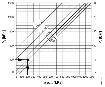
Δp<sub>max</sub> = Differential pressure at a nearly closed valve to largely avoid cavitation
