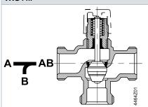
Guided parabolic plug (as of DN25) which is integrated in the valve stem.  $\,$
