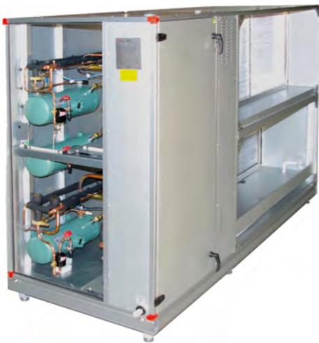
The EQU Q-Cooler is a complete reversible cooling unit designed for cooling the supply air and, alternatively if heating is required, operating as a heat pump recovering heat from the extract air and transferring the heat to the supply air. The cooling unit contains supply and extract air coils, cooling circuits and electrical equipment for power input and safety – all ready-built, wired and tested at the factory.
