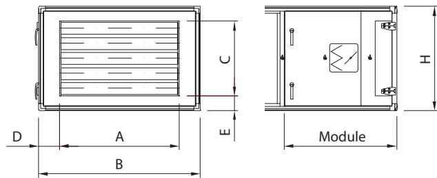
The MIE-ID can be outfitted with deep-pleated, disposable synthetic material filters to class G4, F6 or F7; deep-pleated, disposable glass fibre filters to class F8/F9; deep-pleated carbon filters with integrated pre-filter to class C7 or cleanable knitted aluminium filters. See also the information under the Filter overview tab.
