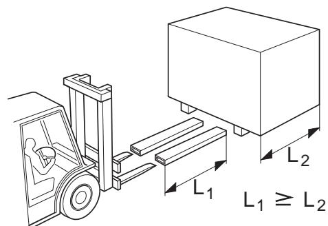
Lifting an AHU with a forklift truck. Make sure that the lifting forks are long enough.
