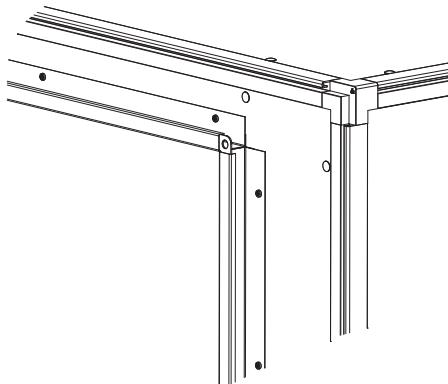
The connections are designed for slip-clamp jointing or for bolted joints in the corners, so-called METU connection.
