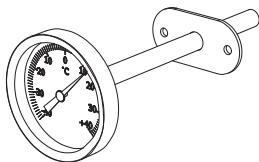
Thermometer of insertion type shown. -40 to +40 °C.
