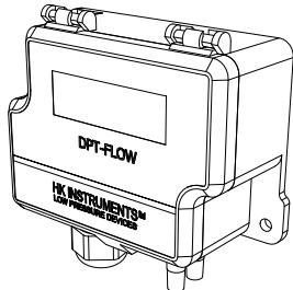
Shows the current airflow. Consists of a display unit and flow-linear pressure sensor. 0-10 V output signal for readings transmitted to an external supervisory system or as a sensor signal for constant flow regulation.
