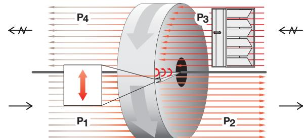
Rotary heat exchangers always carry over a certain volume of extract air to the supply air as they rotate.
