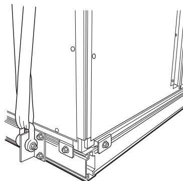
If the AHU is mounted on a support frame it can be lifted using lifting lugs. On an aluminium support frame, the lifting lugs are to be secured with bolts in the grooves provided in the support frame.
