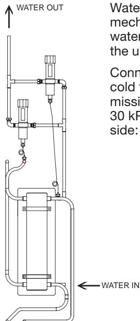
Water-cooled condenser with mechanical pressure controlled water saving valve mounted on the unit.
