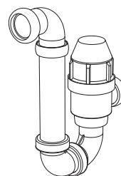
Water trap made of plastic. Built-in non-return valve.
