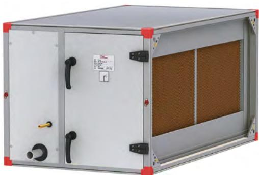
The fitting is selected together with an evaporative humidifier (code EFEF) with cold humidifier fill surfaces which can also be used for evaporative cooling. The fitting consists of humidifier fills, water tray, water distribution system and front casing panel for incorporation into a Standard Module (code EMM).
