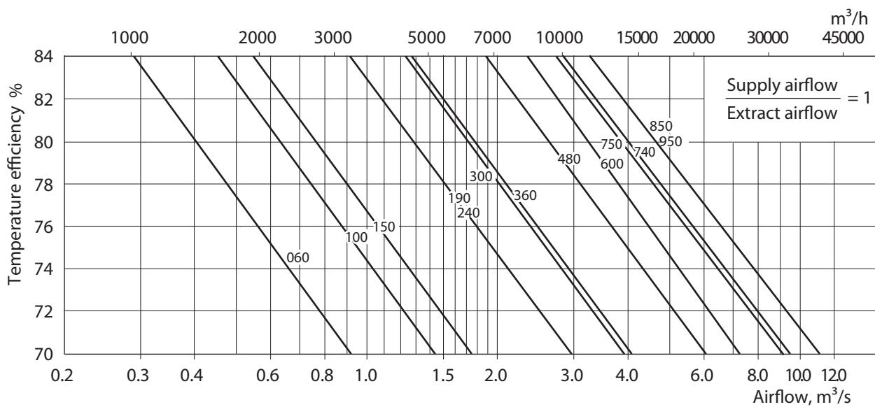
**Temperature efficiency, rotor type NP (Normal Plus) and HP (Hygroscopic Plus)**
