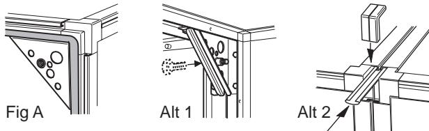
Fit the sealing strip between the unit sections (Fig. A) and joint the sections together with angle brackets and bolts (Alt 1) or slip clamps (Alt 2).
