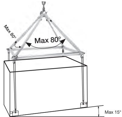
Lifting spreaders should be used for lifting the units.
