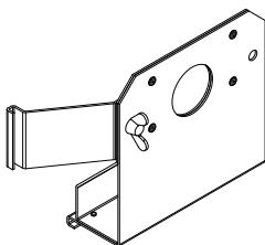
The lifting brackets are designed for insertion into the groove provided in the aluminium profiled frame member. Mount the load safety device and the module is ready for lifting.
