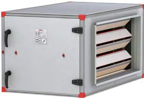
The MIE-ID intake air fitting is designed for the intake of outdoor air or extract air. The fitting consists of dampers, mounting rails for filter cassettes, end connection and front casing panel for incorporation into a Standard Module (code EMM).
