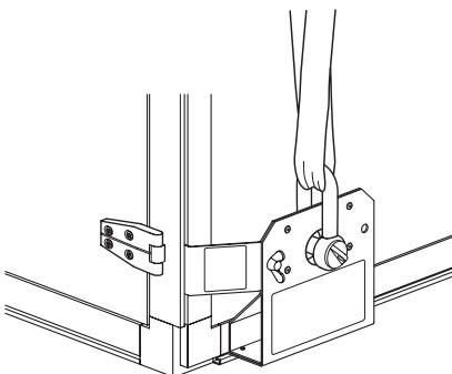
Use lifting brackets for lifting an AHU/Module without support frame (code EMMT-08).
