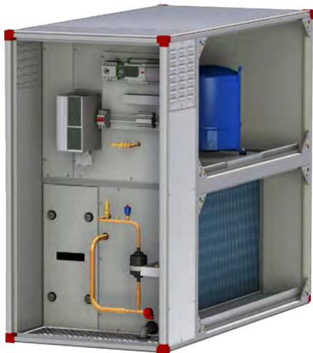
The ACU EcoCooler is a complete cooling unit designed for stepless cooling of the supply air. The cooling unit contains a cooling circuit with evaporator and condenser coils, speed-controlled compressor(s), electronic expansion valves and electrical equipment for power input and safety – all ready-built, wired and tested at the factory.
