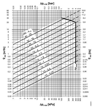
$\Delta p_{max}$  = Maximum permissible differential pressure across the valve (mixing: port A - AB, B - AB),
