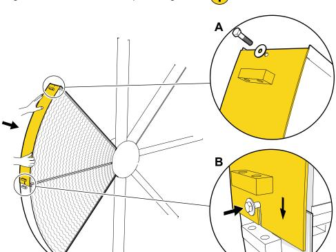
• Fasten the periphery plates together with a clamp bolt. Do not tighten.
