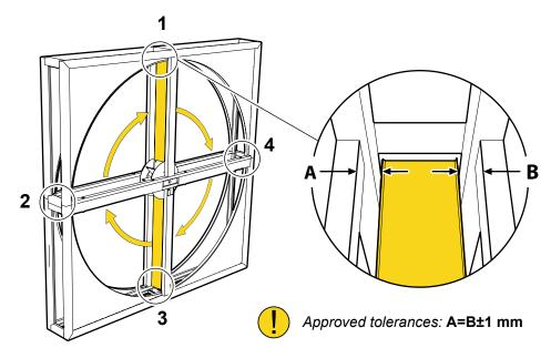
• If the tolerance is not achieved, undo the screw at the wing of the hub and adjust the radial wall horizontally.
