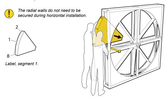
Make sure that the upper and lower edges of the segment are located within the bent edges of the radial walls.
