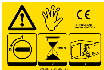
Typical CE label for air handling units
